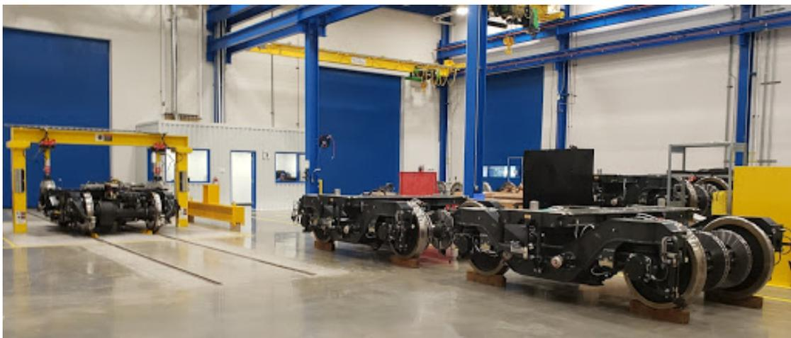
Electric train production continues to ramp up. In July, bogie (truck) manufacturing commenced in the new Salt Lake City manufacturing facility (see above photo). The trucks house the wheels, axles, electric motors, and brakes.
