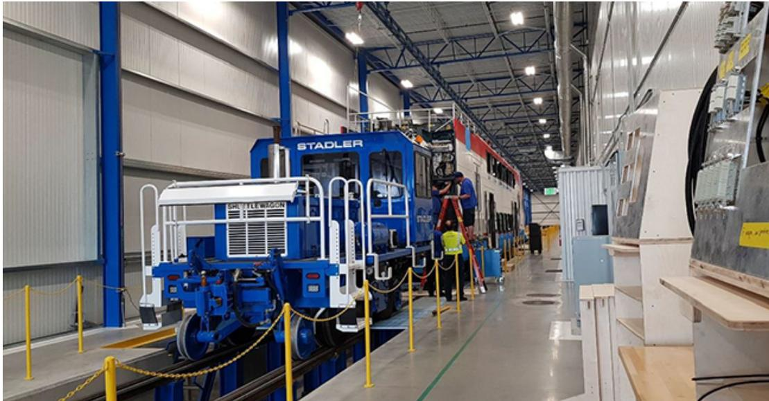
Electric train manufacturing continues to progress. Seat cantilevers and seat racks are being assembled, and two car shells are undergoing preliminary electrical testing (as seen above). There are now 19 cars in the final assembly stage, and manufacturing on car shells for trainset #4 has commenced. To view more photos visit [CalMod.org/gallery](http://CalMod.org/gallery).
