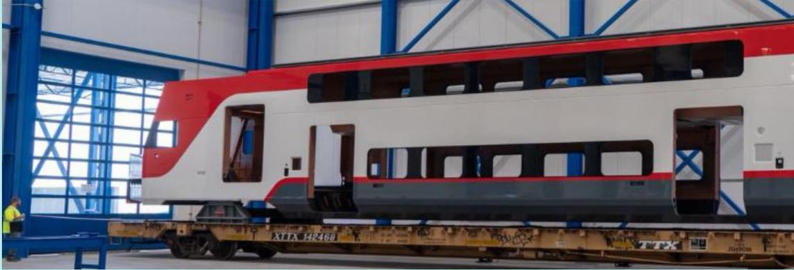
In December, electric train manufacturing made progress with the start of conduit and thermal insulation installations in four carshells of Trainset #1. Testing and inspections of the electric train systems such as HVAC, doors, seats, couplers, and friction brakes also continues.
