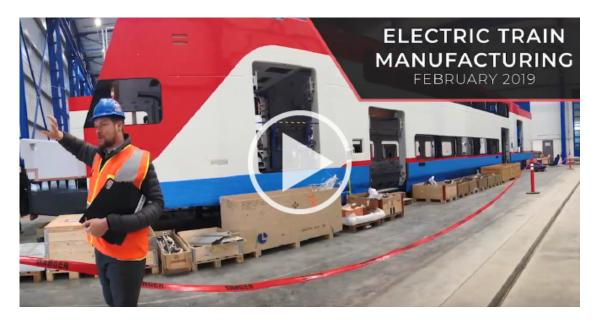
Interior equipment installation is now occurring in six of the car shells! Check out the video to see the upper level floors take shape in the primed car shells, as workers install mounting brackets and flooring. First article inspections continued in February, along with static and fatigue testing.
